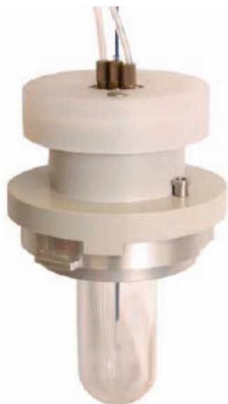
Figure 2. Voyager head unit, reaction vessel and fibre optic probe in thermowell.
